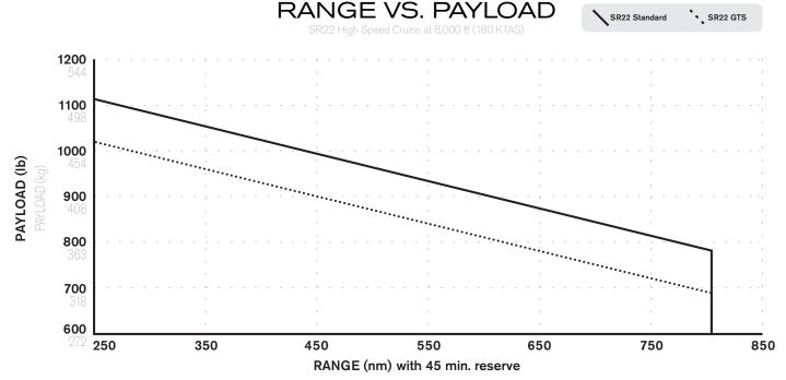
+1 lb (.45kg) Payload or Equipment = -1.7 NM 75% to 55% PWR = +40% Range
