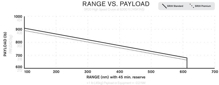
(.45 kg) Payload or Equipment = -2.2 Ni 65% to 55% PWR = +8% Range
